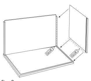
Step 2: Apply glue inside the corner moulding on the back wall and along the bottom edge of a side wall; slide it into the channel in the side of the base.
