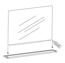
Step 4: Remove the protective backing from the acrylic pane. Apply a thin line of glue along the bottom edge only and position the pane in the center of the channel at the back of the frame trim. Hold pane upright until the glue sets.
